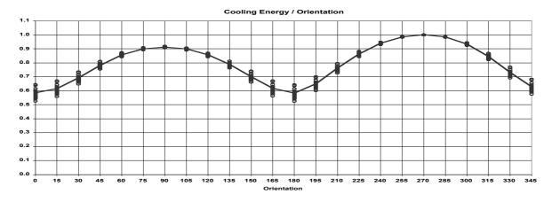
Figure 2. Energy necessary to cool the offices for various building orientations
