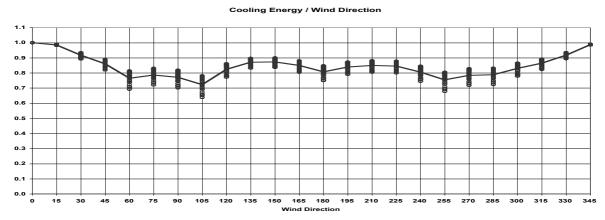
Figure 3. Energy necessary to cool the offices for various wind directions
