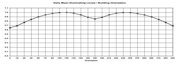
Figure 4. Daily mean illuminating levels for various building orientations
